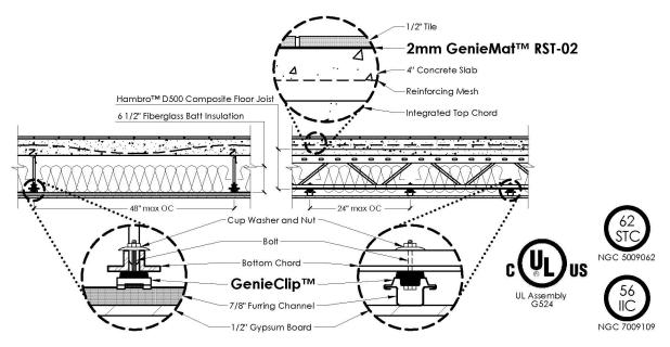
Exhibit C – Published IIC Laboratory Test Scores of Hambro System – ceiling mounted with GenieClips.
